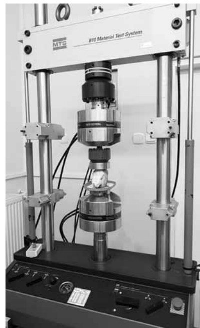
Fig. 2. A research site used for fatigue testing of the joints
