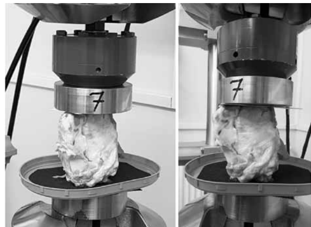
Fig. 16. The joint in the fatigue testing machine holders (sample No. 07): a) before the test, b) after the test
