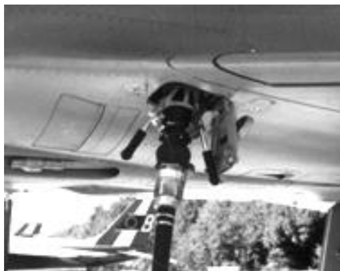
Fig. 2. Refuelling of the aircraft with a pressure head
