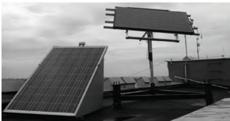
Fig. 8. View of measurement stand to determine the annual distribution of power density of solar radiation, taking into account changes in the spatial orientation of the receiver PV
