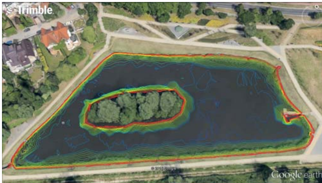
Fig. 14. Isometric projection of the retention reservoir in Gdansk with the marked coastline and contour lines (own study)
