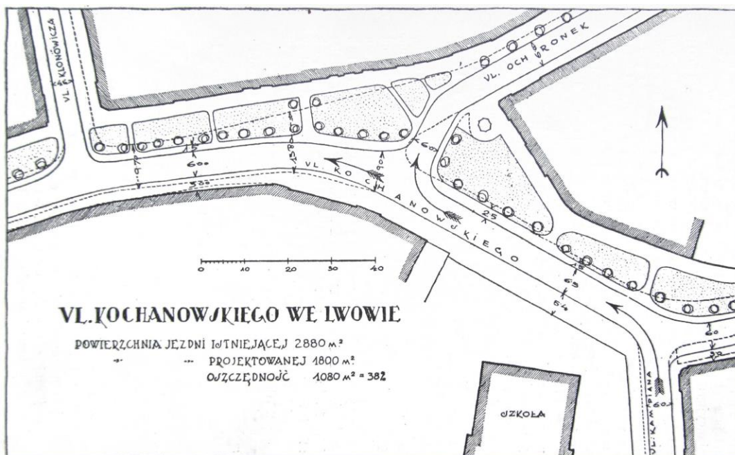
Fig. 7. I. Drexler's arrangement of Kochanowski (today - Levytskoho) street, 1928. Due to the width narrowing of the driveway part of the street up to 6 m and change of the radii of turns into the side streets, 38% of the street space was saved for other needs - the sidewalks were expanded and lanes with green islets from the northern side of the street were formed, where they received the necessary insolation. Source: I. Drexler [6].
