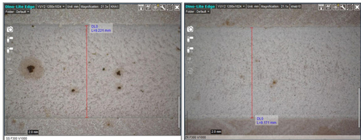
Fig. 7. Maximum groove lengths after machining the cuts from f = 0.03 mm/tooth and s = 1000 m/min SS316 (left) and ZrO_2 (right)
