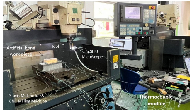
Fig. 2. Milling operational set-up with thermocouple module and In SITU Microscopic camera
