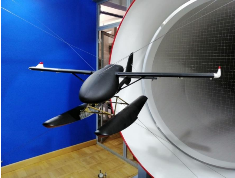
Photo 1. The “OSA” with floats installed, suspended in the wind tunnel test section.
