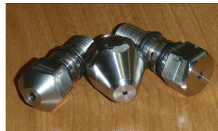
Fig. 2. STK air-and-water spraying nozzles (Prostański 2011b)
