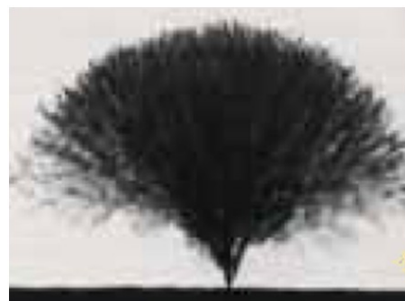
Fig. 6. View of water treeing in polyethylene insulation of a cable [8]
