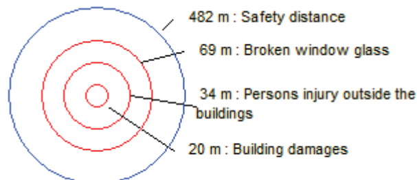
Fig. 2. Consequences of the explosion of 7.5 kg TNT. Terex was used for this assessment
