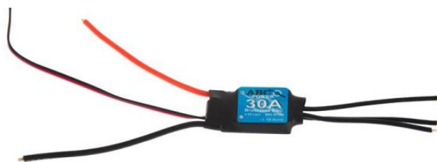
Rys. 7. Regulator obrotów ABC-Power 30 A [10]
