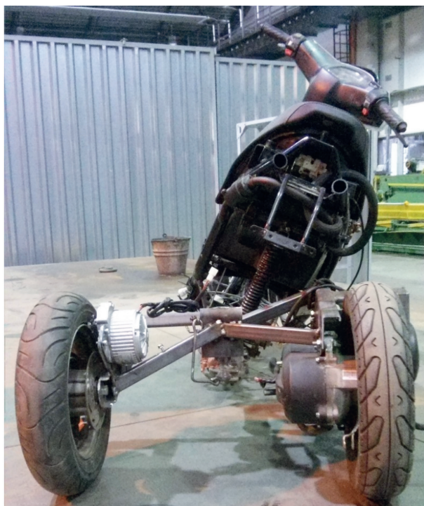
Fig. 5. The second prototype of the three-wheeler in the position of maximum tilt of the vehicle body [source: authors' materials]
