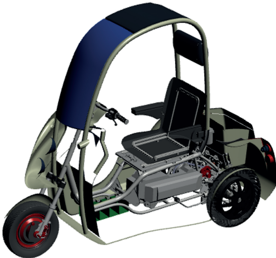
Fig. 2. CAD model of the three-wheeled invalid carriage with an independent rear wheels suspension system [source: authors' materials]
