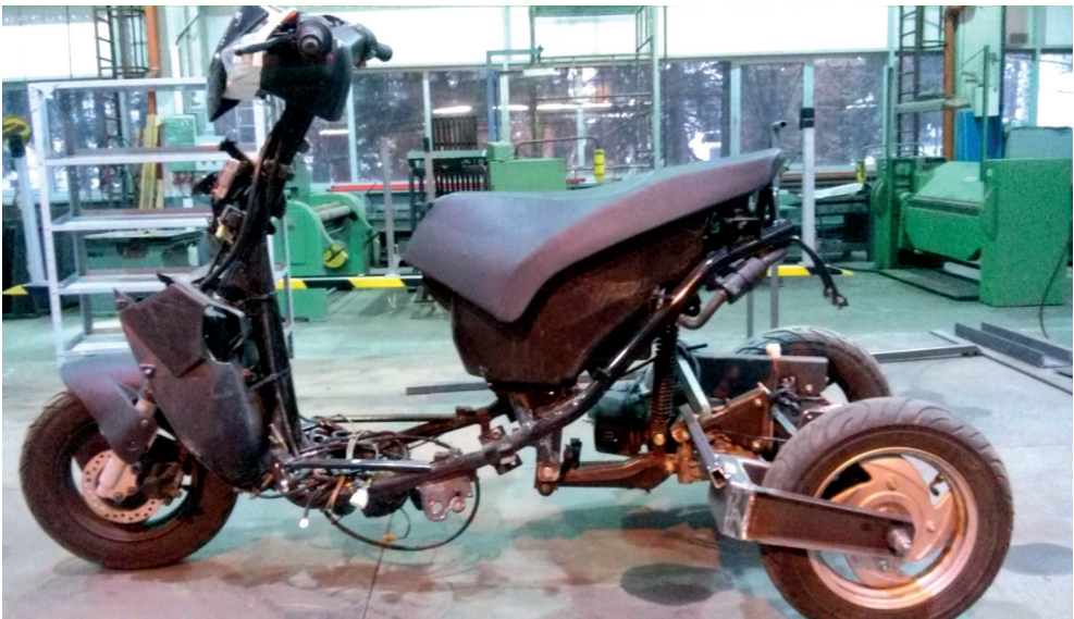
Fig. 3. The second prototype of the three-wheeled invalid carriage, with the dependent rear wheels suspension system [source: authors' materials]
