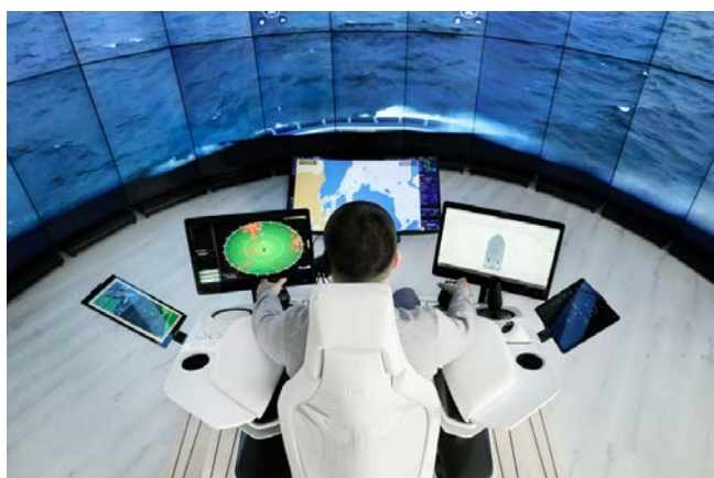
Figure 2. Remote operation station for autonomous ship, note nautical chart displayed [8]
