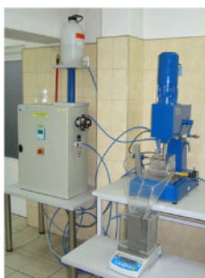
Fig. 3. Stand for testing the flotation process [32]
