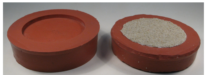
Fig. 3. Molds made from silicone rubber
