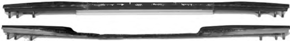
Fig. 1. View of exploited carbon contact strips: a – worn out, b – totally damaged
