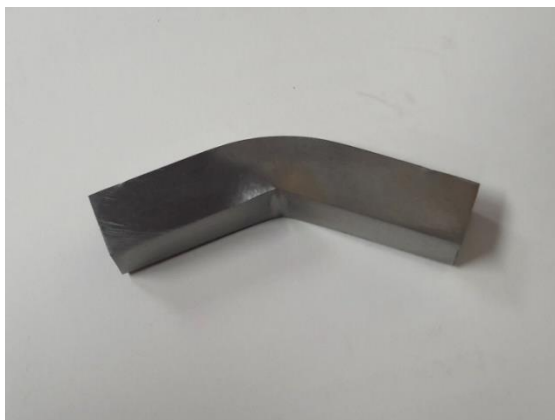
Fig. 2. Overview of an unbroken specimen following a hardness test with a ram at the initial energy of 300 J.
