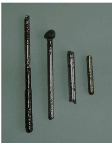
Fig. 9. Exemplary cast rods prepared using the furnace with the suction attachment
