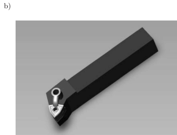
Fig. 4. Chipformer 23 measured geometry a) and assembled tool [6] b).
