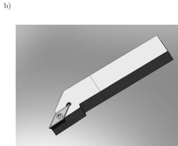
Fig. 5. Chipformer SM measured geometry a) and assembled tool [6] b).
