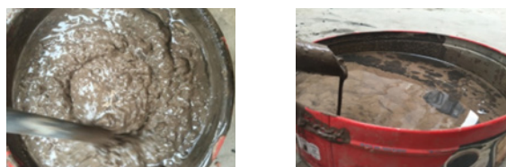
Fig. 7. Results of transport experiment in the pipeline: a. ratio of fly ash 18% < b < 30%, b. b < 18% và b > 30%
