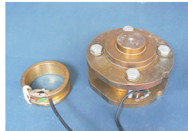
Fig. 9. An oedometer for the measurement of lateral stresses, constructed at IBW PAN
