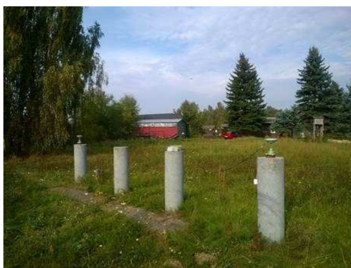
Fig. 12. Points of GNSS field calibration test baseline at WUT Józefosław Observatory
