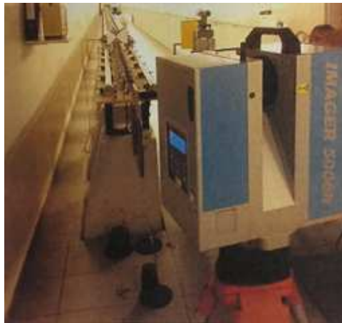
Fig. 23. Position of scanner relative to interferometric comparator
