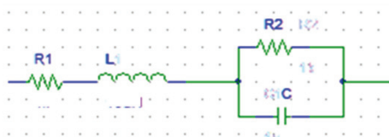
Fig. 6. Supercapacitors: a) view of fabricated product; b) equivalent circuit of a supercapacitor
