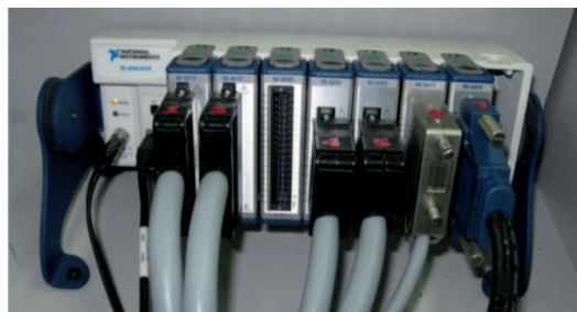
Fig. 4. NI data acquisition boards integrated as CompactDAQ system
