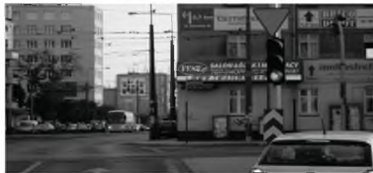
Fig. 3. An example of an LED billboard located right in the driver's line of sight, also being a false background for traffic lights
