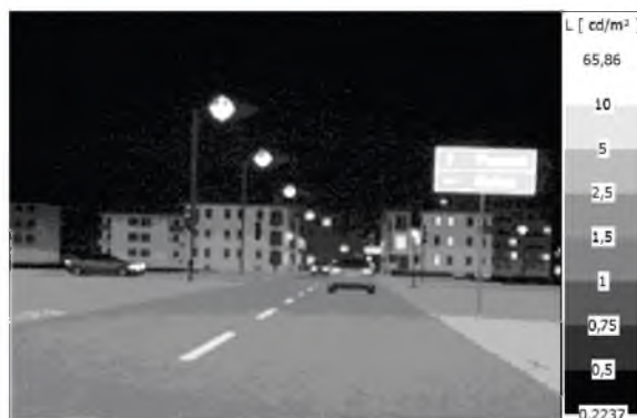
Fig. 6. Distribution of luminance in the displayed section of the road and in its direct vicinity
