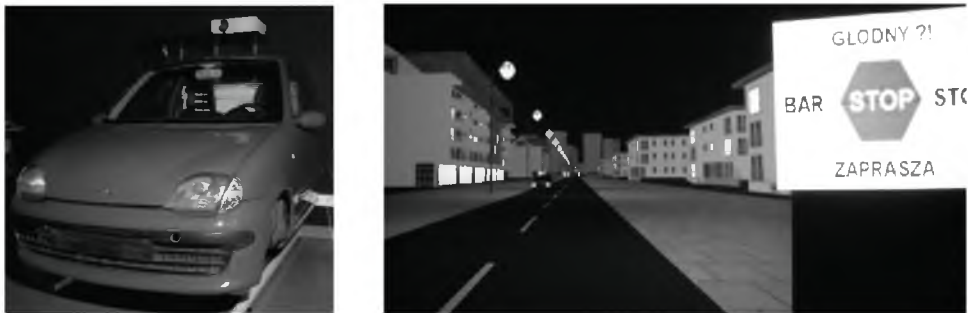
Fig. 4. The road simulator on the left, the working LED billboard and the vehicle simulator on the right
