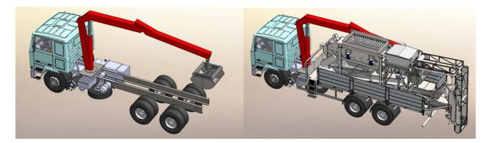
Fig. 3. Used Iveco lorry on the left and EB50 mixer mounted on the Iveco truck on the right
