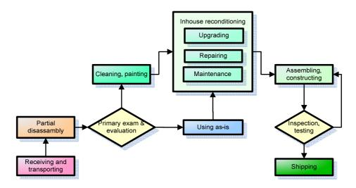
Fig. 4. The process of bringing used Iveco lorry to new life
