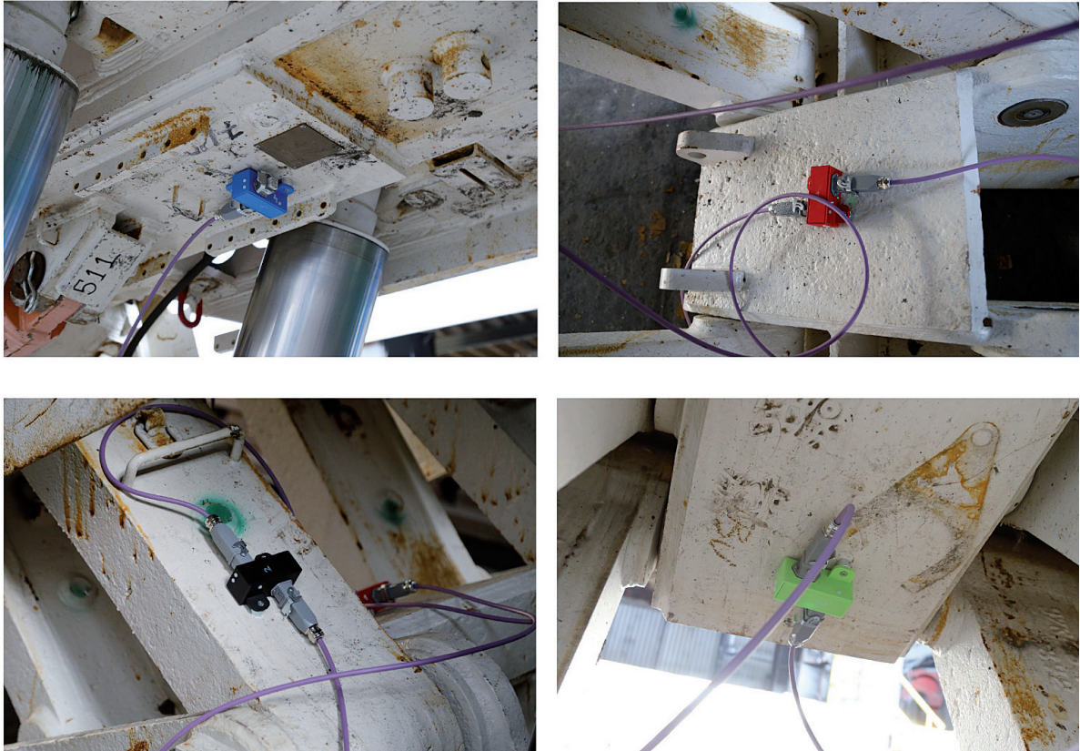
Fig. 6. Places of the inclinometers installation: a) canopy, b) base, c) lemniscate link, d) gob shield
