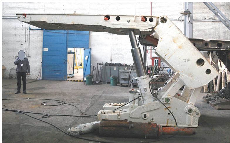
Fig. 5. JZR 13/28 POZ shield support
