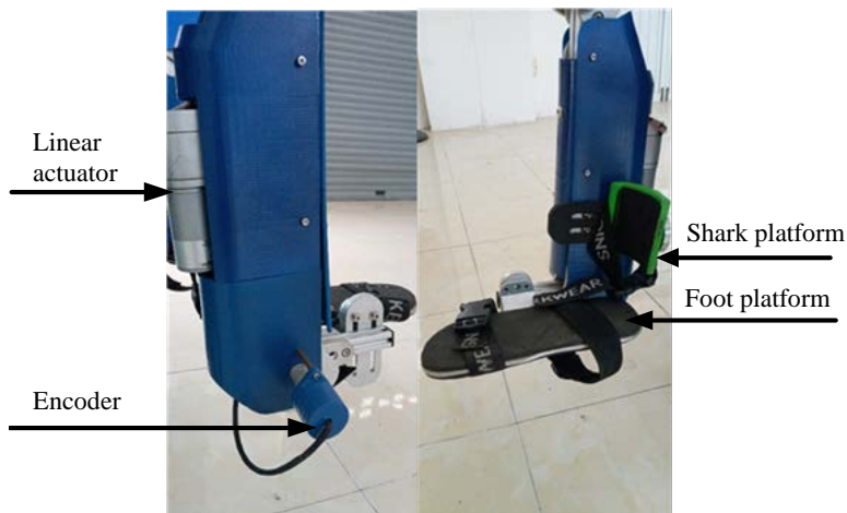
Fig. 7. Prototype of the ankle rehabilitation device
