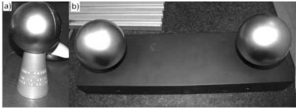
Fig. 10. Standards for acceptance tests for: a) probing error, b) sphere-spacing error [23].
