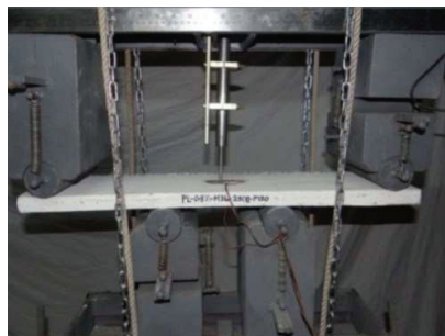
Fig. 2. Flexural Test Set-up (with test specimen)
