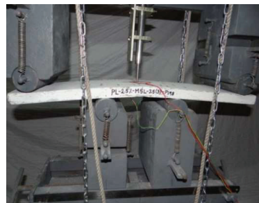
Fig. 10. Deflection Ductility of 5E
