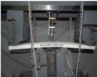
Fig. 9. Deflection Ductility of 5D
