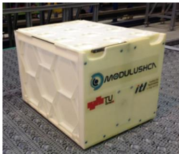
Fig. 2. Prototype of the modular logistic unit
