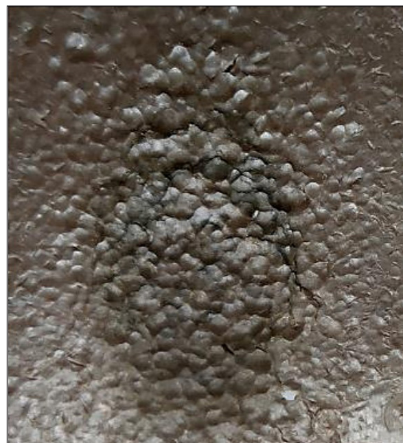
Fig. 8. Photograph of the surface of the sample with model contamination after treatment with a pulsating jet of liquid with metal balls, angle 125° (scale 1:3)
