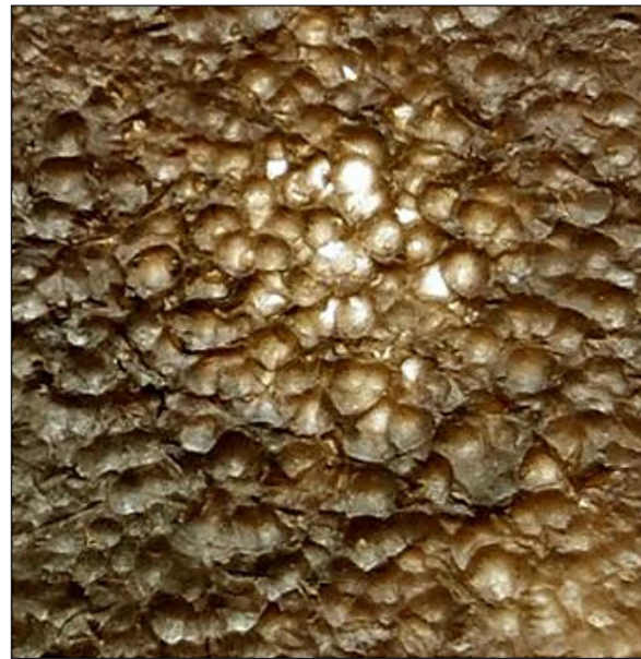
Fig. 7. Photograph of the surface of the sample with model pollution after treatment with a pulsating jet of liquid with metal balls, angle 90° (scale 1:8)
