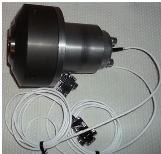
Fig. 4 Sensor for measuring the cutting force F_s
