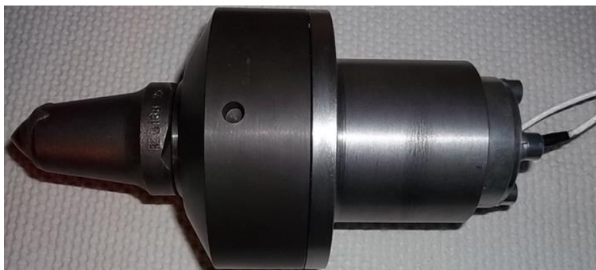
Fig. 3 Measuring head body with measuring blade
