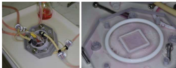
FIG. 1. Cultivation chamber for dynamic endothelisation of decellularized pericardium connected to perfusion system and sterile ports (left), fixed decellularized tissue in chamber (right).
