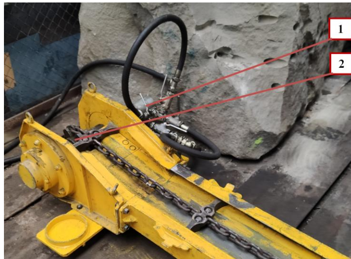
Fig. 3. Stand for testing dynamic forces – view from the drive wheel side, markings: 1- hydraulic motor, 2- drive wheel
