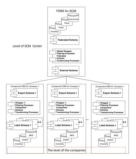
Figure 2. The architecture of Federated Database Systems in Supplies Chain Management
