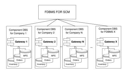
Figure 1. Federated Database Systems and its components
