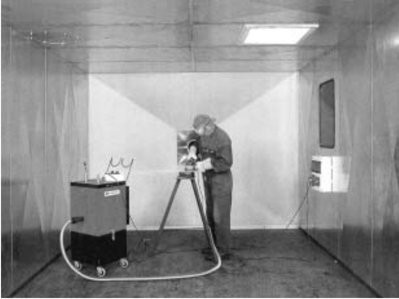
Figure 1. Test stand for determining the efficiency of emission reduction for suction components of local exhaust ventilation during measurements for a manual power sander connected to a filtrating-ventilation unit.
