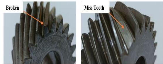
Fig. 14. Broken and missing teeth in the pinion gear
