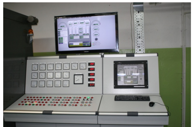
Figure 4. Laboratory stand for the measurement and analysis of indicator graphs
