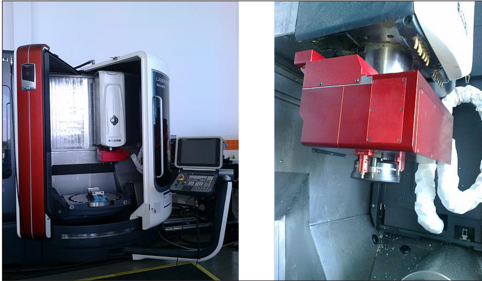
Fig. 2. Machining station – LASERTEC 65 Shape SAUER machine tool
