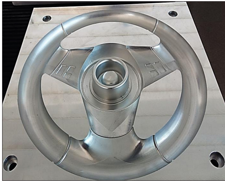
Fig. 1. Object of machining – semi-finished die of the steering wheel of a wheeled motor vehicle
