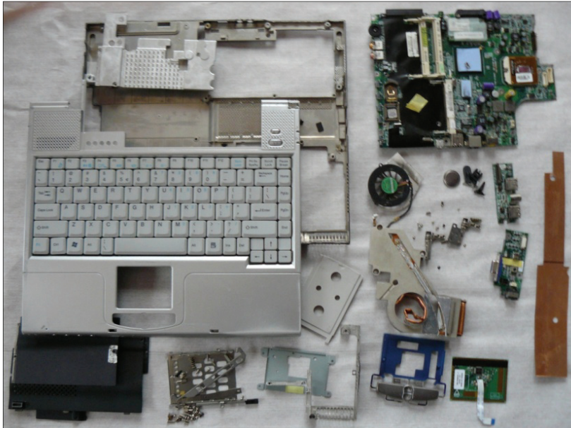
Fig. 3. Dismantled housing of the laptop, all main components are visible [20]
