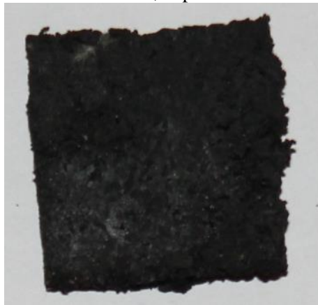
Fig. 2. Rubber-poliurethane sample designed to tests with TPMU method
