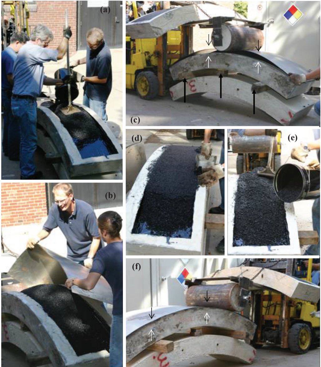
Fig. 3. Stages of the TPTA pavement sample compaction process: (a) first stage: pre-densification, (b) specimen before the first stage of compaction, (c) first stage: compaction, (d) removing mixture covering top of the concrete mold, (e) second stage: pre-densification and (f) second stage: compaction
