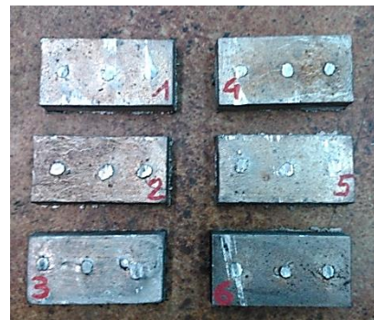
Fig. 2. Plates surfaces; 1 - Koalid 2290, 2 - WV-Coating 401 200, 3 - PV-Coating W220, 4 - Dimanol Al, 5 - Tellurschlichte 813
