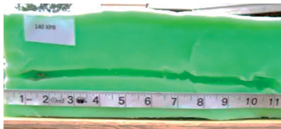
Figure 3. Ballistic soap after a shot photo by Jason Wimbuscus ( www.guns.com/news/2017/06/16/think-of-all-the-fun-you-could-have-with-backyard-ballistic-testing-materials )
