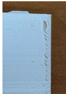
Figure 22. Melting of the outer surface caused by overheating (e.g., due to too long or frequent stay of the printing nozzle head in the same area).
