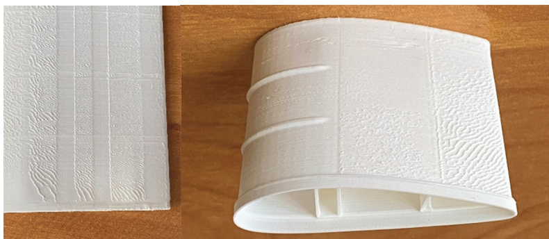
Figure 20. Waves caused by the non-extrusion movement of the printing nozzle.
