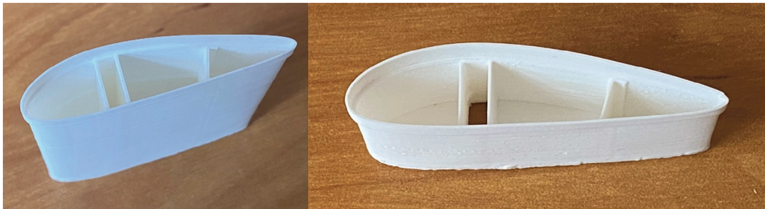
Figure 12. Printed segment of a wing with positioning collar that is used for final assembly.
