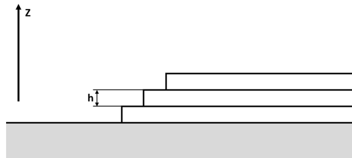
Figure 7. Print layering in the Z direction.
