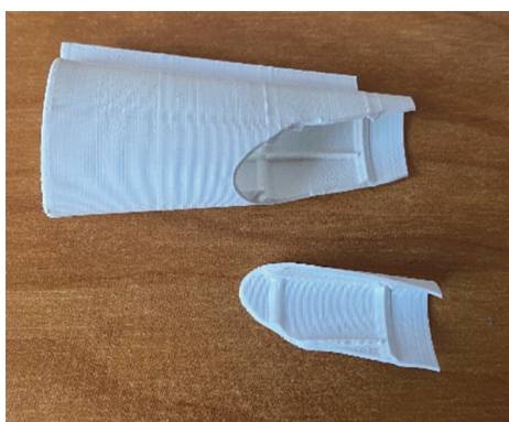
Figure 5. Section of a typical semi-monocoque structure of a fuselage. FDM, fused deposition modeling.
