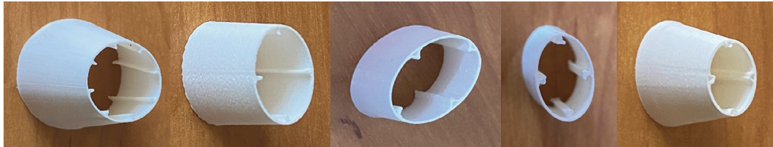
Figure 14. Elements strengthening the fuselage structure.
