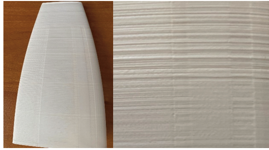
Figure 21. Collapse of the shell caused by the presence of elements reinforcing the semi-monocoque structure.
