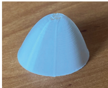
Figure 19. Print defects: limitations for prints without supports and a seam resulting from a temporary stop of the printing head on its path.
