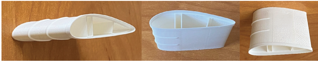
Figure 16. Embossing on the leading edge.
