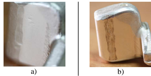
Fig. 2. Silver plated copper switch-disconnector main contacts; new (a) and worn (b)
