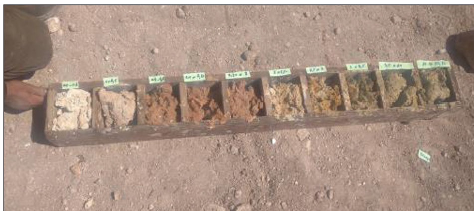
Fig. 3. Wooden box containing the geological formations of the borehole
