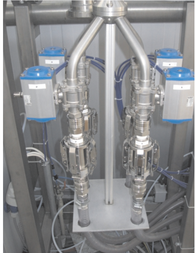
Fig. 5. Particulate sampling system for PM measurements
