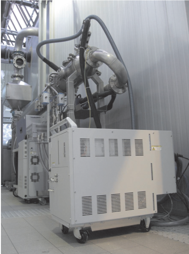
Fig. 3. Dilution tunnel (looking upstream) and HORIBA 2000-SPCS PN counter (foreground)
