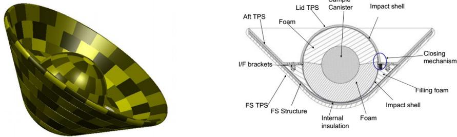
Fig. 1. Earth Re-entry Capsule design for Earth Re-entry Demonstrator mission [2]
